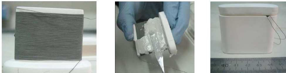
Fig. 2 A first layer of insulated Ni wire is wound around an alumina core, an insulation layer of MgO is applied. After a second layer of wire is wound, the casing is closed and sealed.
