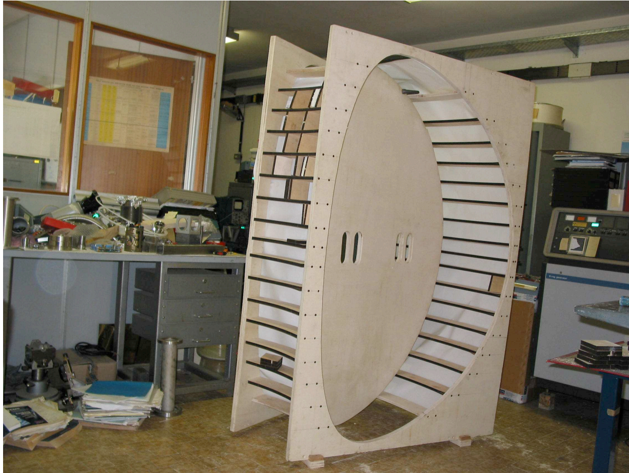
Full size wood model of one sector of the Ignitor plasma chamber.
