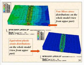
Comparisons of the results obtained for two physical quantities in the numerical simulations of MF1 and MF2 models , as concerns TIG-Ng welding
